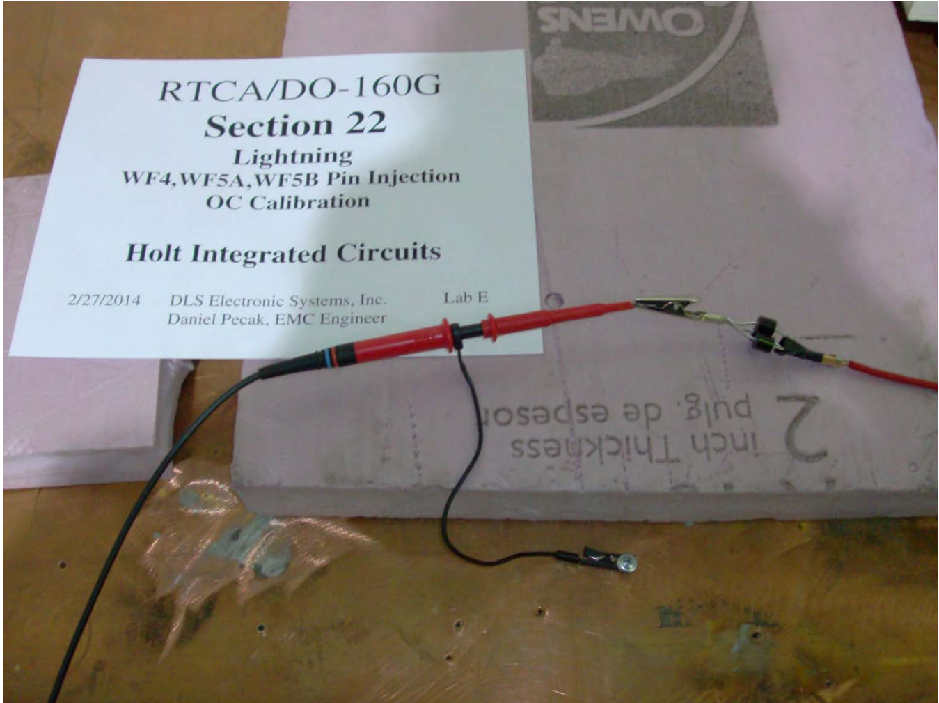
Section 22 Pin Injection - WF4, WF5A & WF5B OC Calibration
